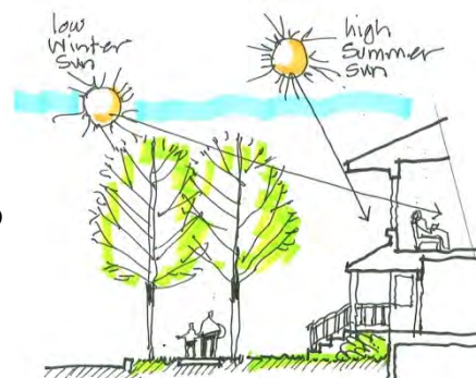
Figure 62. Ensure light penetration into interior living spaces in winter, and protection from direct sunlight in the afternoon hours of summer.
