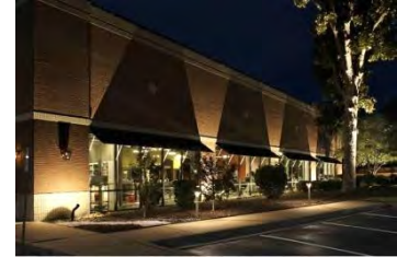
Figure 77. A combination of wall-mounted lights and up lighting animate the building façade and adjacent pedestrian areas.
