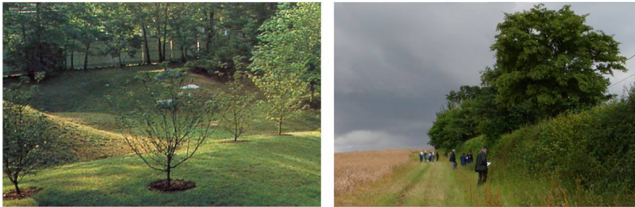
Figure 11. Earthen berms and hedgerows are two noise mitigation strategies employed at the DDA site.
